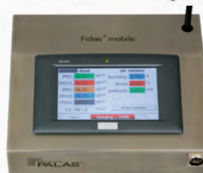
FIDAS mobile (Palas) PNC, size-distr. (32K/Dekade) 0.2-18 \mu m PM 10/4/2.5/1
