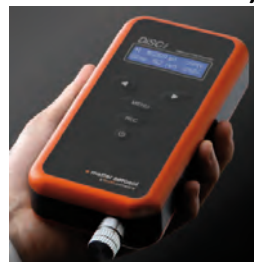
DiSCmini (Matter Engineering) PNC/LDSA(alveo.) 10-300 nm modal
