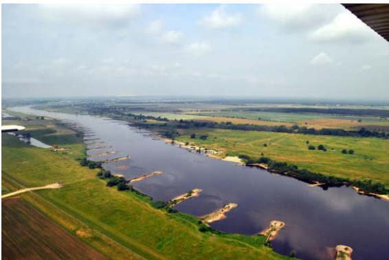
Massive bank protection: groynes
