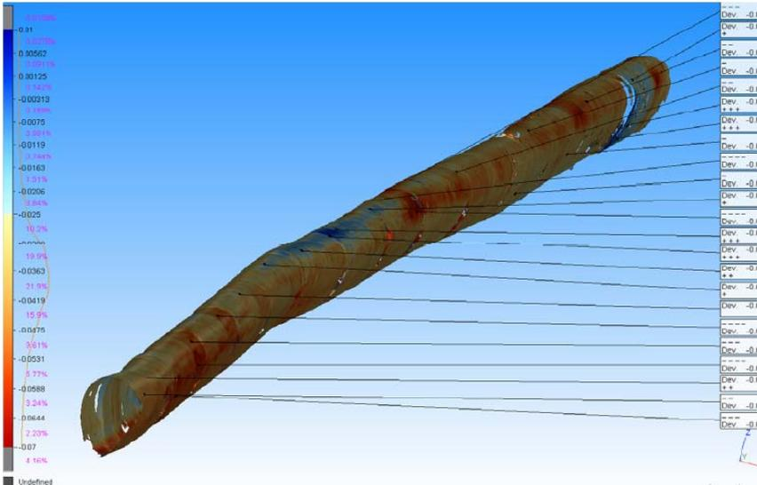
Abb. 51: Deformationsanalyse (Software 3DReshaper) [108]
