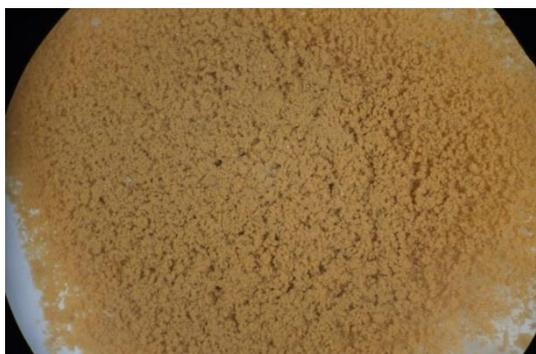
Emfloc KA 3; 0,5 g<sub>FM</sub>/kg<sub>TR</sub>
