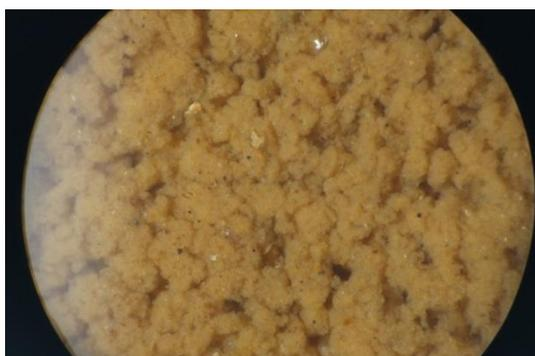
Emfloc KA 3; 0,5 g<sub>FM</sub>/kg<sub>TR</sub>
